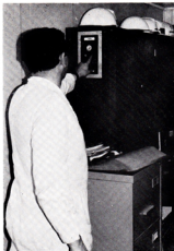
■ Engine room machinery alarms are transmitted via a master control panel to all engineer officers' cabins in King Alfred . Above: A. Russell, chief engineer officer, checks the master control panel in his office while . . . see below . . .
