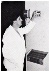
■ . . . on the receiving end of a call, L. Ord, senior second engineer officer, accepts an alarm condition in his cabin before proceeding to the engine room to deal with the fault.
